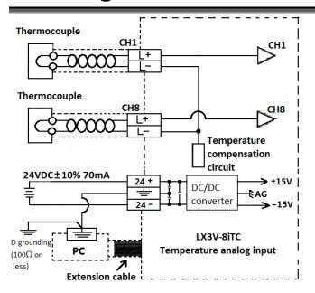
(1) The temperature compensation cable connected to thermocouple is as follows:
