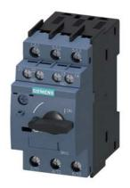
Circuit breaker size S00 for motor protection, CLASS 10 A-release 0.45...0.63 A N-release 8.2 A screw terminal Standard switching capacity with transverse auxiliary switches 1 NO+1 NC
