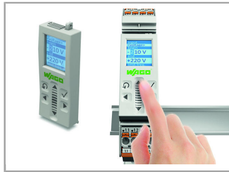
Configuration via WAGO configuration display
