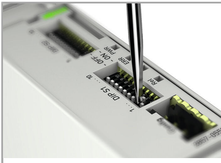
Configuration via DIP switches
