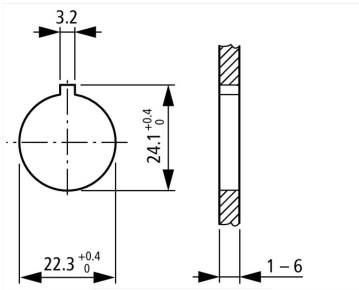
Mounting hole with lug slot
