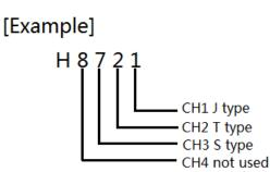
The time of A/D conversion is 240ms for each channel. When "3" (unused) is set for a channel, this channel would not have A/D conversion, therefore, the total time for conversion decreases. In the above example, the conversion time is as follows:
