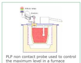
Precimeter non contact measuring systems - withstanding over 800°C; suitable for aluminium, magnesium, lead, tin, zinc. Other materials are available on request.
