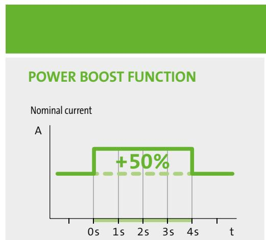
The Current Limiter and Power Limiter functions are excellent for starting capacitive loads. Units with these features do not simply switch off, but they reduce the voltage or provide a higher inrush current with the PowerBoost function.
