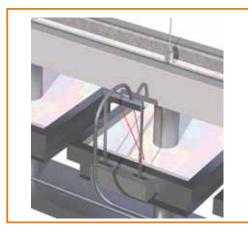
The ProH Mould Edition sensor is, amongst other applications, very suitable in slab casting applications for mould level control.
