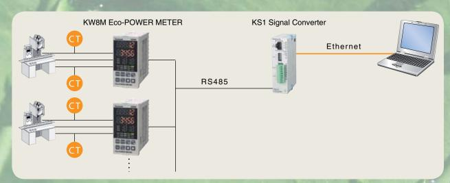
Every Eco-POWER METER is equipped with an RS485 interface for easy and cost-efficient networking. KS1 Signal Converters allow integration into any Ethernet network.
