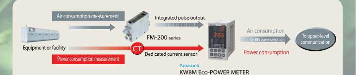
The SUNX Digital Flow Sensor FM-200 allows you to save energy and costs in other ways, e.g. by measuring how much air is consumed in industrial processes. You can even connect the FM-200's pulse output to the Eco-POWER METER's pulse input to measure air consumption and power use simultaneously.
