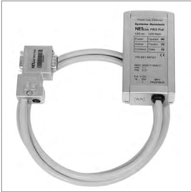
NETLink® PRO PoE, PROFIBUS Ethernet gateway
