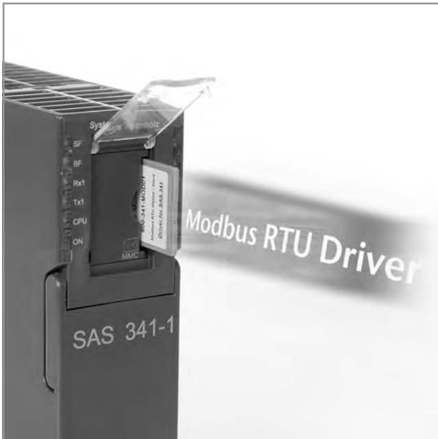
SAS 341-1 with Modbus RTU driver
