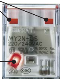
Relay with AC Coil (LED: Red)
