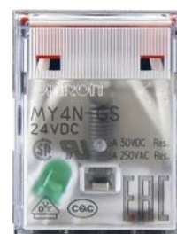
Relay with DC Coil (LED: Green)
