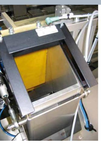
Slot grid sensors handle challenging counting and monitoring tasks such as detecting non-guided objects in free fall.
