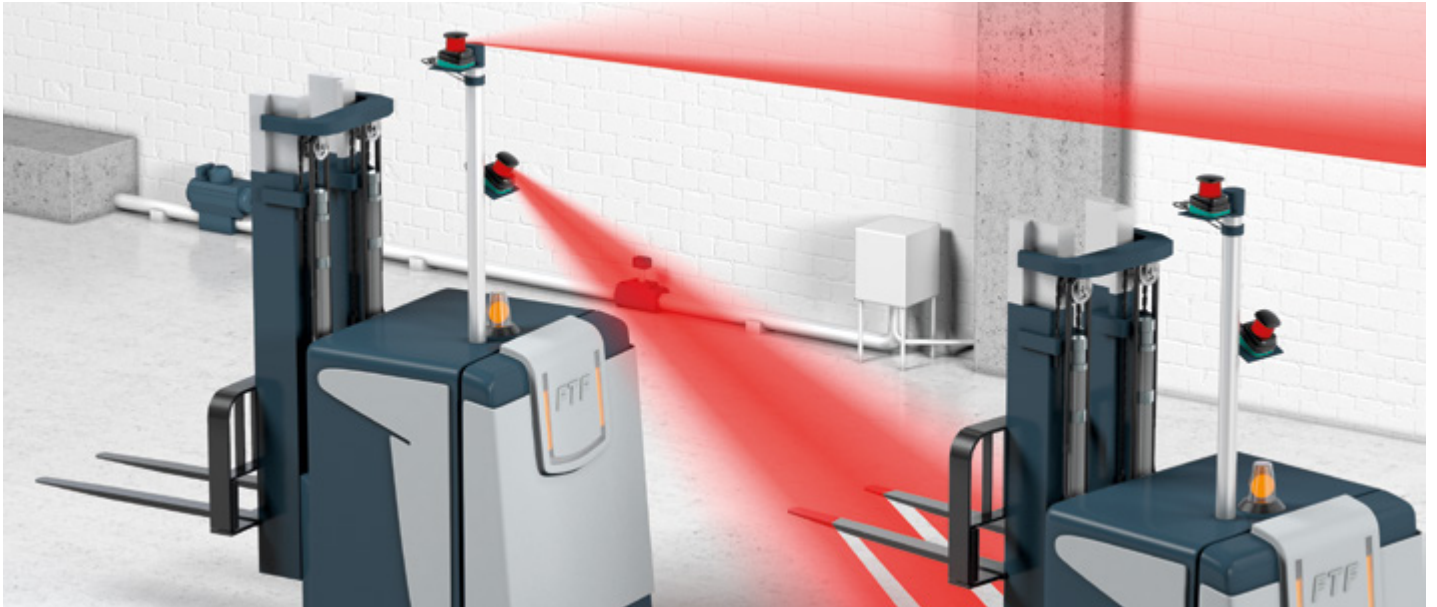
R2000 UHD provides distance, angular, and signal data for navigation
